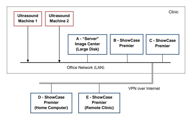
The Ultrasound Machines send study data to the **A** "Server" computer running ShowCase Image Center. The Image Center stores the study data to a large disk. ShowCase Premier on computers **B** and **C** is configured to access the Image Center directly, as local viewers. ShowCase Premier on computers **D** and **E** are configure to access the Image Center over a VPN, as remote viewers. The Image Center will store up to 200,000+ studies.
